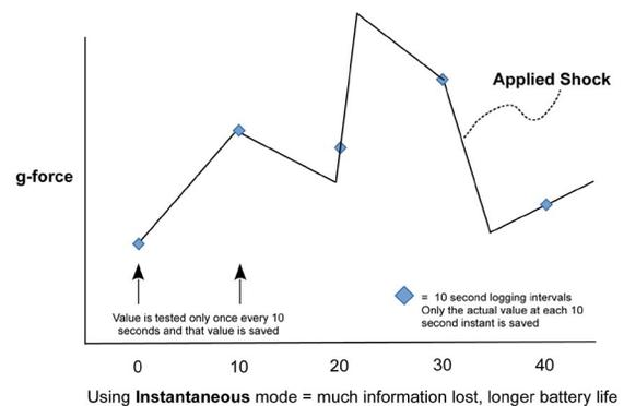
The potential to lose valuable data can be seen. This, of course, is very dependent on the applied shock duration and wave shape. It's possible for a significant shock event to occur and not even be visible in the data for the Instantaneous mode.
