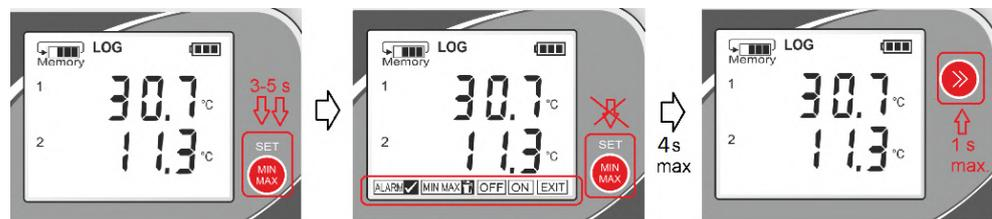
You can now work with individual menu items. Press the upper key to scroll through the menu items, press the lower key to confirm (SET). After confirming certain choices, the menu will be quit automatically. If the keypad is inactive for more than 20 s, the menu will close automatically.
