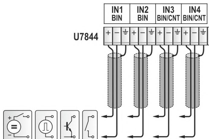
For the procedure for connecting wires to the connecting block refer to Annex 4.
