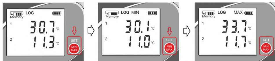
The device can also be set up to toggle the „screens“ automatically, in for about 5 sec interval. The cycle can be interrupted by pressing a key. If you do not want to use the keypad, you can disable it in the device settings.
